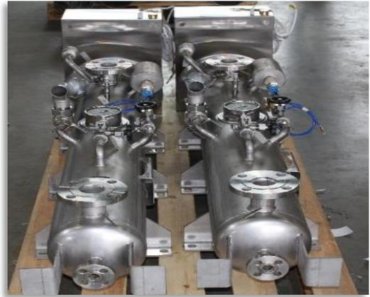
Vertical brake resistors delivered to Transocean.
