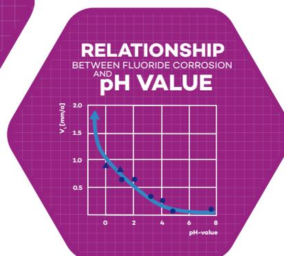
Corrosion progress V<sub>L</sub> in relation to pH value; in a solution with 19 mmol/l Fluoride at 80 °C.
