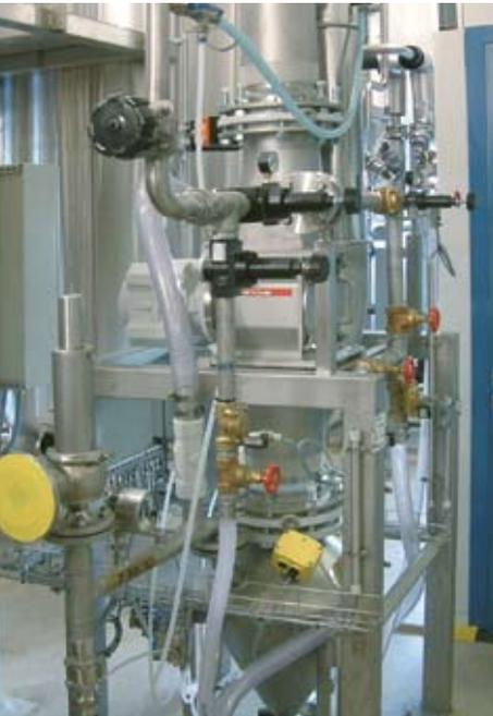
NBS 200/200 installed before pneumatic dense phase conveying
