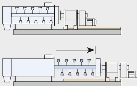
mixer is moved to cleaning position on a guide rail
