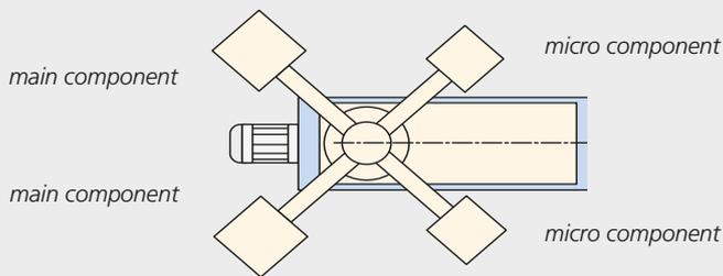
loading circular layout of metering units
