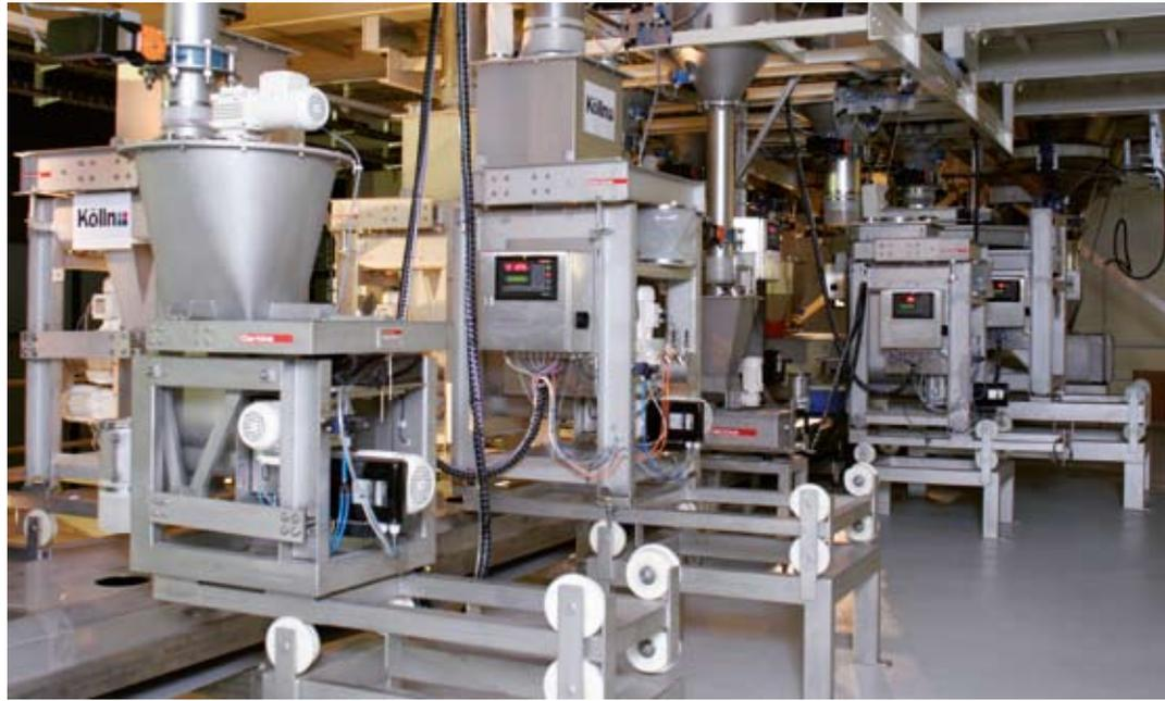
The correct placement of feeders and mixers makes safe operation and cleaning easier.
