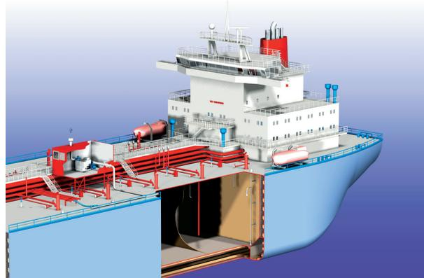
AG-S tank dryers provide efficient drying and reduced lay-time for chemical tankers.
