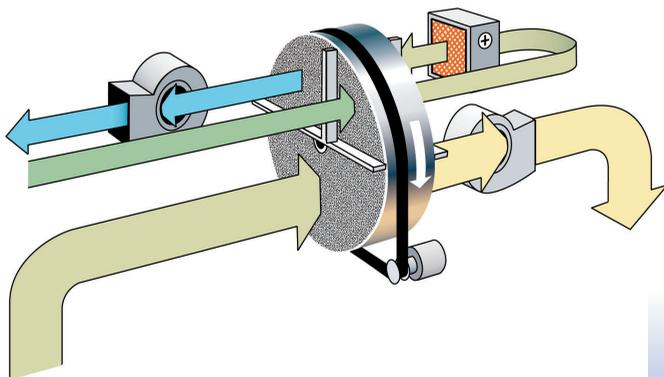
AG's maritime dehumidifiers are based on the Recusorb principle: Efficient drying at all relevant temperatures, also below 0 °C.
