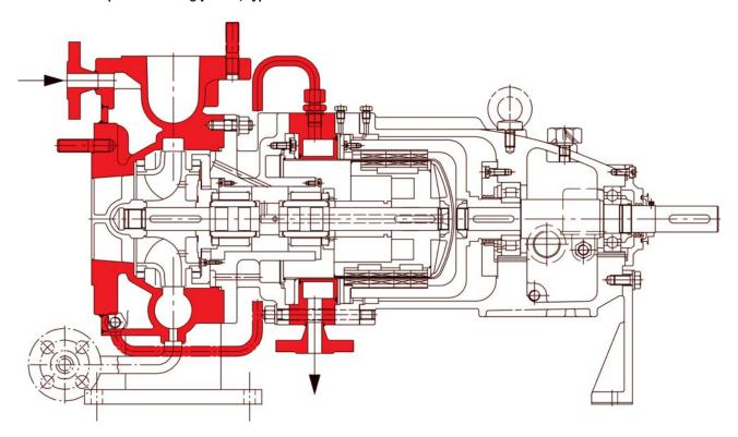
For handling fluids with melting temperature above ambient. Design data for heating jacket 24 bar / 250°C (485°F).
