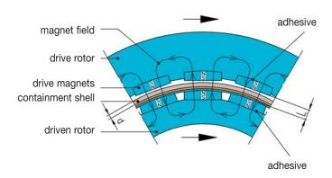
The couplings are designed to transmit rated motor power up to 220 kW (295 hp) at 2900 rpm, respectively 260 kW (348 hp) at 3500 rpm.
