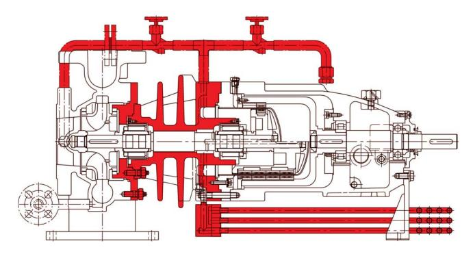
For handling heat transfer fluids up to 400°C (750°F) the PRMW-design with air cooler reduces the fluid temperature in the magnet area to maximum 250°C (485°F) and keeps away dirt and pipe scale from the magnetic coupling.
