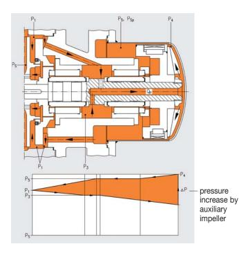
The cooling flow is led from the discharge side behind the impeller into the chamber between the slide bearings and through the pump shaft via the auxiliary impeller again to the discharge side. This design pressurizes the slide bearings and the containment shell with nearly the full discharge pressure and the product remains stable in this area.
