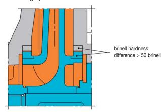
Mating wear surface materials have a difference in Brinell hardness of at least 50 HB.
