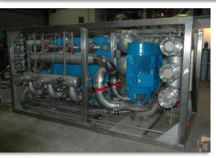
Seawater/freshwater buffersystem with leackage detection and automatic emergency filling. Three units delivered to Odfjell
