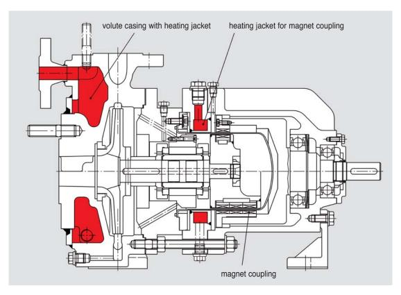
Type KMR - with oil lubricated bearing bracket
