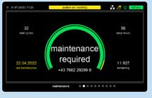
Complete transparency and tracking of maintenance-critical factors such as lamp hours, start cycles and maintenance intervals
