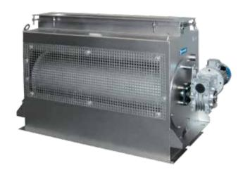
The CER line is one of the two iron remover product lines offered for CER 600-900-1200 powders. It is composed of a drum made of neodymium permanent magnets. It posseses an automatic cleaning system. It is ideal for processing large quantities of materials.
