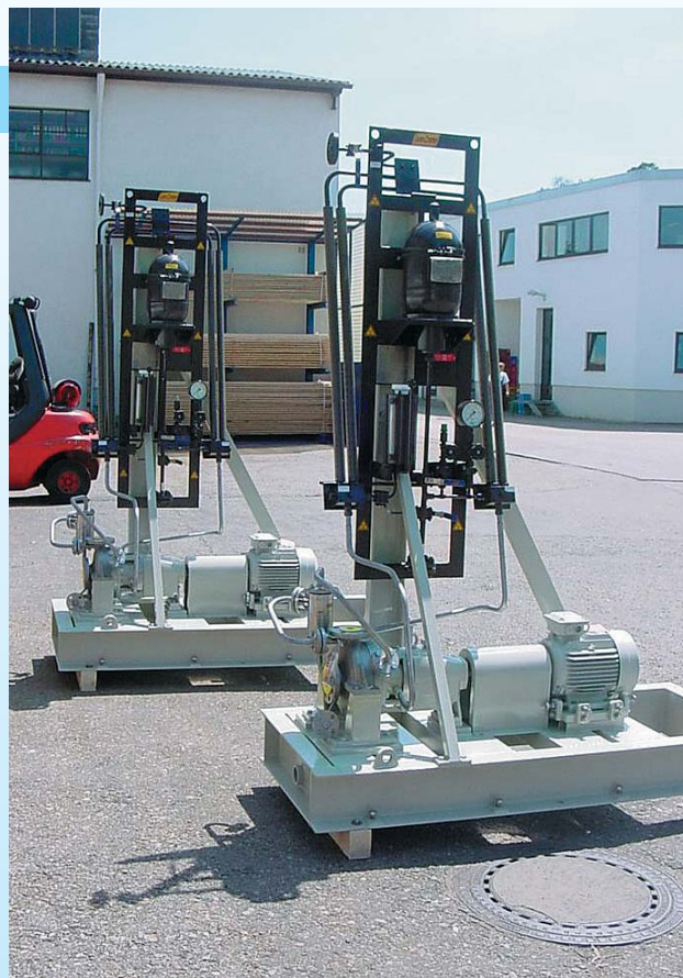
Type NCR – API 610 9th ed. with double seal system plan 53B + 31. Liquid: Aqueous Hydrocarbon (offshore application).
