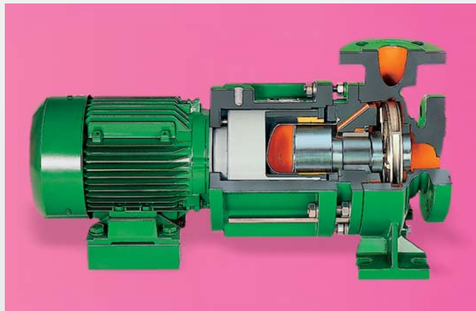
Volute casing pumps type KMB with hermetically sealed magnetic coupling. Capacity up to 60 m 3 /h (300 USgpm), differential head up to 60 mLC (300 ft).
