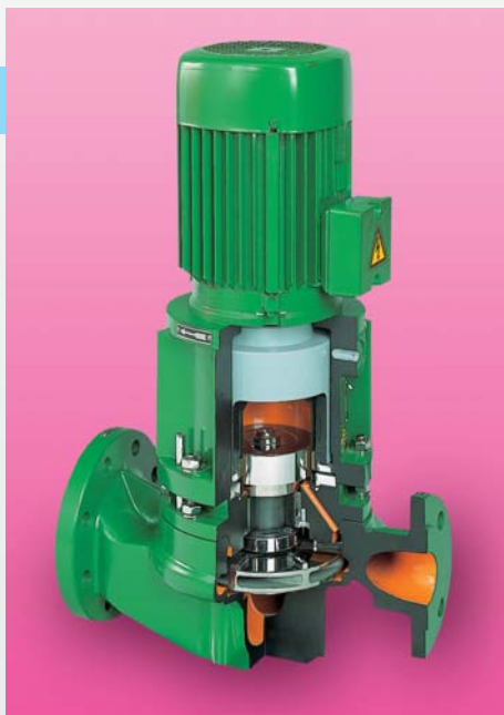
Inline-volute casing pumps type KMV with hermetically sealed magnetic coupling. Capacity up to 60 m 3 /h (300 USgpm), differential head up to 60 mLC (300 ft).
