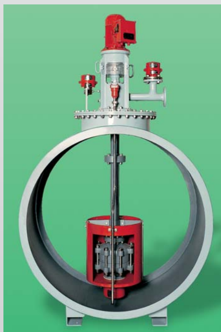
Multistage centrifugal pumps type HZSMA with gas handling stage on pressure side and hermetically sealed magnetic coupling.
