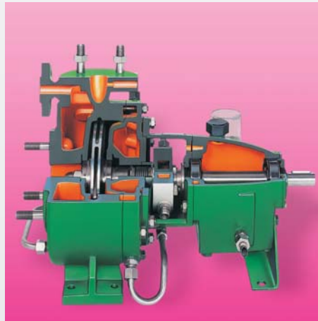
Volute casing pumps type NCLb with heating chamber on suction and pressure side, and heated single mechanical seal N6b.
