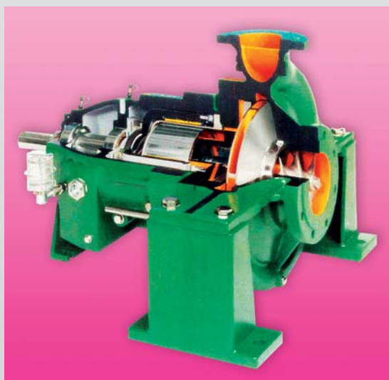
Volute casing pumps type PRM acc. to API 685, with hermetically sealed magnetic coupling, centerline mounted
