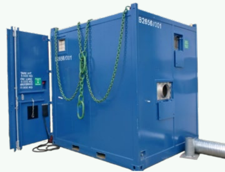
10ft AG-EXC-082E with 4,500 m 3 /h dry air, for zone 1
