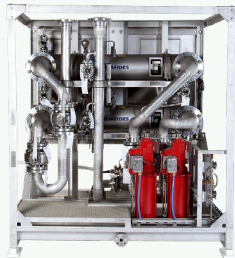
UV skid at Oseberg C
