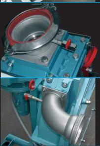
Delivery fitting complete of air pressure or nitrogen nipple
