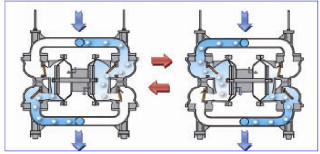
Top suction / bottom-discharge design keeps solids from settling in pump
