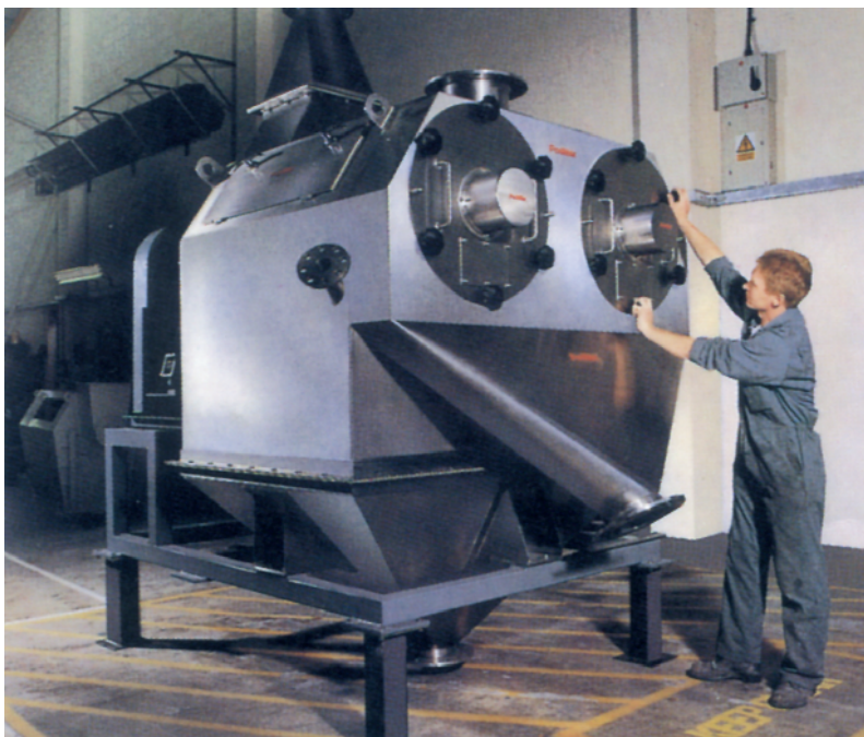
Special CSM 1542 Twin Sifter on final assembly
