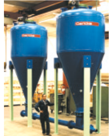
Continuous conveying of fly ash at 130 m 3 /h with double sender.
