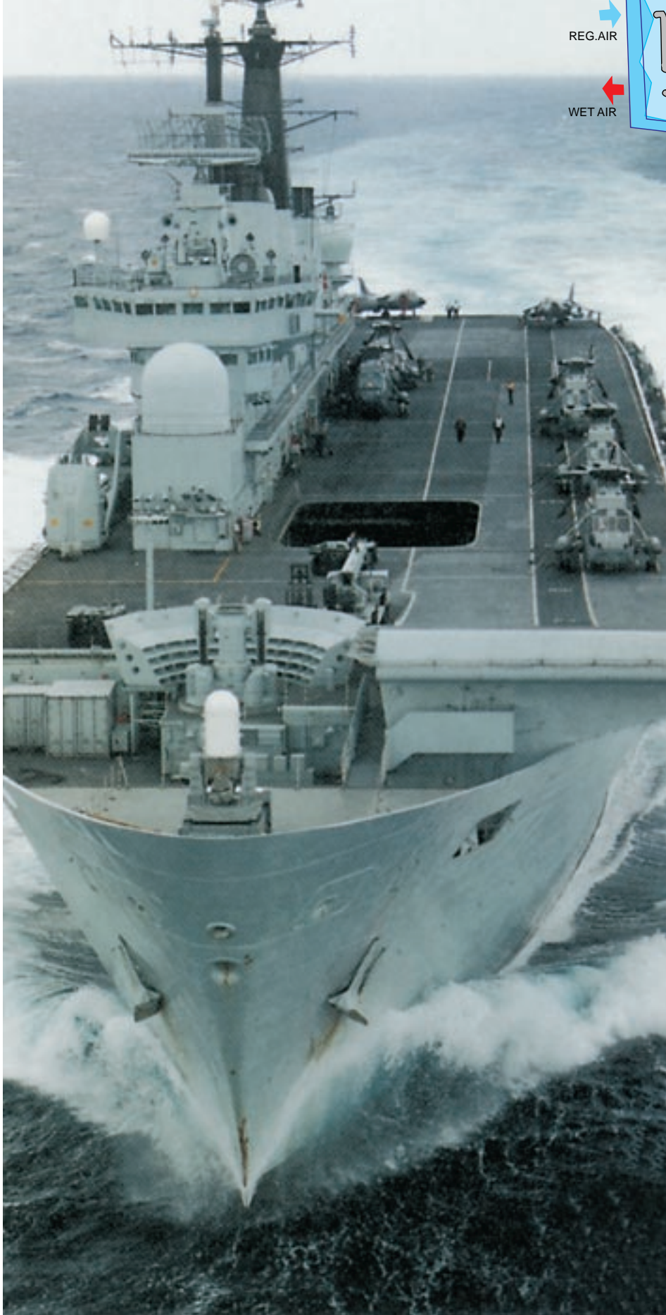
HMS Ark Royal, United Kingdom, is, until it's due for a new commission, kept in a state of extended readiness by 29 DST dehumidifier units. (Photograph by the courtesy of the Ministry of Defence, U.K.)
