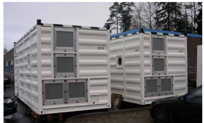
Climate container with a dry-air flow of 4,500 m 3 /h, delivered to Bilfinger
